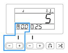
Each press of "-" makes the zigzag stitch narrower.
