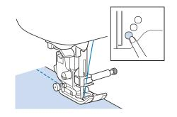
$\bigcirc$  Press the 3 (Thread cutter button) to trim the upper and lower threads.
