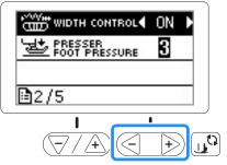
$\rightarrow$  The machine is now set so that the stitch width can be controlled with the sewing speed controller.
