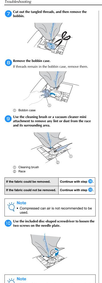
Be careful not to drop the removed screws in the machine.
