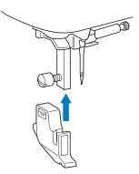
Hold the presser foot holder in place with your right hand, and then tighten the screw using the screwdriver in your left hand.
