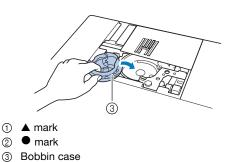
• Make sure that the indicated points are aligned before installing the bobbin case.
