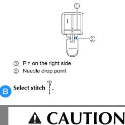
• When using zipper foot "I", be sure to select the straight stitch (center needle position), and slowly turn the handwheel toward you (counterclockwise) to check that the needle does not touch the presser foot. If a different stitch is selected or the needle hits the presser foot, the needle may bend or break.
