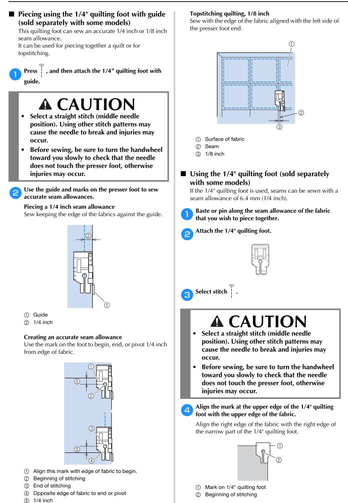
When sewing with a seam allowance, align the left edge of the narrow part of the 1/4" quilting foot with the fabric edge.
