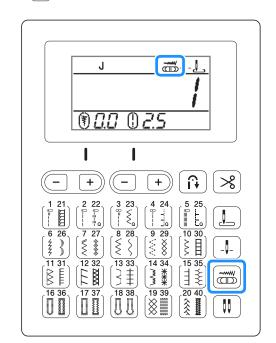
$\rightarrow$  The machine is now set so that the stitch width can be controlled with the sewing speed controller.
