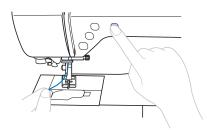
→ The bobbin thread is looped around the upper thread and can be pulled up.
